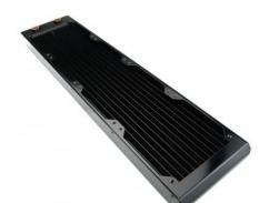
HX-CU1320VS is a low profile copper core radiator designed for four 120mm fans. With a fin density of 20 FPI (fins per inch), it is optimized for quieter air flow ranges. It has a dual pass coolant design, and is G 1/4 BSPP (parallel) thread for hose fittings. 30mm (1.18") long mounting screws are included for 25mm thick fans (see Koolance <u>radiator screw packs</u> for additional options).
