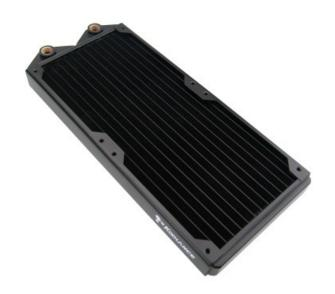
The copper core HX-CU-1402V is designed for two 140mm fans. With a high fin density of 30 FPI (fins per inch), it offers best performance at higher air flow. Vertical (perpendicular) G 1/4 BSPP (parallel) thread fitting sockets, dual pass, 30mm (1.18") long mounting screws included.
