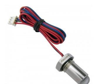
Koolance infrared liquid level sensor. Total length of sensor = 29mm (1.14in). Nickel plated brass, G 1/4 BSPP threading.
