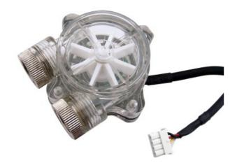
Koolance's inline flow meters provide electronic indication of real-time coolant flow rate. Internal LEDs can be illuminated with optional components described below. This model uses a reed switch to detect impeller rotation. G 1/4 BSPP fitting threads, and primary materials are nickel-plated brass and acrylic. Approximate read range is 0.5-15 LPM (7.8-238 GPH). Wire length is approximately 19" (48cm).
