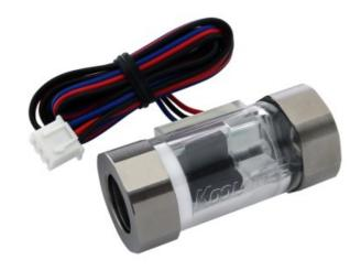
Koolance's inline flow meters provide electronic indication of real-time coolant flow rate. This model uses a hall effect sensor to detect impeller rotation speed. G 1/4 BSPP fitting threads, and primary materials are nickel-plated brass and acrylic. Approximate read range is 1.0-20 LPM (15.6-317 GPH). The flow meter accepts 4.5-24VDC, and a maximum current of 10mA. Wire length is about 28" (70cm).
