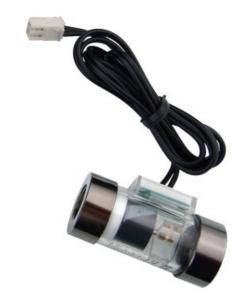
Koolance's inline flow meters provide electronic indication of real-time coolant flow rate. This model uses a reed switch to detect impeller rotation. G 1/4 BSPP fitting threads, and primary materials are nickel-plated brass and acrylic. Approximate read range is 1.0-20 LPM (15.6-317 GPH). Wire length is about 28" (70cm). It is recommended to keep current through the flow meter at 10mA or less to prevent damage.
