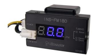
INS-FM18D combines an LCD display with Koolance's stainless steel flow meter in a small footprint. The display shows flow rate in liters per minute (LPM) only. A 12VDC connection is required for power. Primary materials are a stainless steel body with nickel-plated brass G 1/4 BSPP threads.
