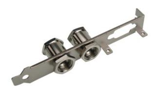
Dual panel-mounted socket threads for "internal/external" fittings on a computer chassis L-bracket. The female G 1/4 BSPP threaded couplings can be removed from the L-bracket and used as panel-mountable unions. Nickel-plated brass. This product may need to be temporarily disassembled during installation.
