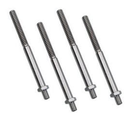
Threaded mounting posts for the Koolance CPU-390, CPU-380, and CPU-370 to fit socket LGA-1366 processors with a fixed motherboard back plate. These four bolts screw directly into the stock motherboard back plate using an M3 thread.
