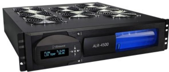
ALR-4500 is Koolance's highest performing ambient liquid cooling system. It can be oriented in horizontal or vertical orientations, and is rack-mountable. This model contains a large eight x 120mm fan copper/brass radiator, providing roughly 4600W of cooling with a 25°C ambient delta. Coolant flow rate, temperature, and reservoir level are monitored, and a USB port allows control and logging of most features using the [Koolance System Monitor](#) application.
