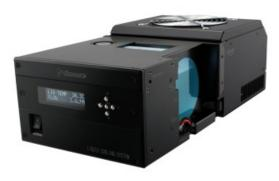
ALX-750-P400 contains a one-fan copper/brass radiator, providing about 750W of cooling with a 25°C liquid-ambient delta. Coolant flow rate, temperature, and reservoir level are monitored, and a USB port allows control and logging of most features using the <u>Koolance System Monitor</u> application.
