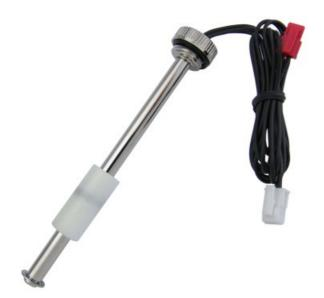
Koolance liquid dual level sensor with column float and two 2-pin connectors. Circuits are normally open until float reaches the middle (red connector) and bottom (white connector) of the metal column. Total length = 100mm. Nickel plated brass, G 1/4 BSPP threading.
