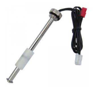
Koolance liquid dual level sensor with column float and two 2-pin connectors. Circuits are normally open until float reaches the middle (red connector) and bottom (white connector) of the metal column. Total length = 100mm. Nickel plated brass, G 1/4 BSPP threading.
