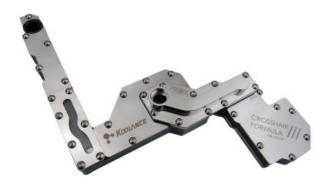
The MB-ASC3F water block is designed exclusively for the ASUS Crosshair III Formula motherboard. It liquid cools the northbridge chipset and other nearby components. Materials include copper with anti-corrosive nickel plating, acetal body, and an acrylic and steel top cover. G 1/4 BSPP fitting threading.
