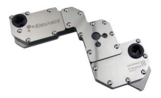
The MB-ASM3F water block is designed exclusively for the ASUS Maximus III Formula motherboard. It liquid cools the northbridge chipset and nearby components. Materials include copper with anti-corrosive nickel plating, acetal body, and an acrylic top with steel plate cover. G 1/4 BSPP fitting threading.
