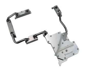
The MB-ASP6T7WS water block is designed exclusively for the ASUS P6T7 WS SuperComputer motherboard (not included). It liquid cools the northbridge, southbridge, and voltage regulators using fixed copper pipe and blocks. Materials include copper and brass with anti-corrosive nickel plating. G 1/4 BSPP fitting threading.
