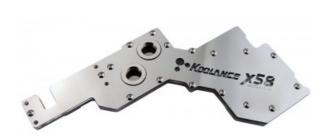
The MB-ASR2E water block is designed exclusively for the ASUS Rampage II Extreme motherboard. It liquid cools the northbridge and southbridge chipsets, along with nearby components. Materials include copper with anti-corrosive nickel plating and an acrylic top. G 1/4 BSPP fitting threading.
