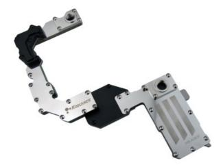
The MB-ASR3F water block is designed exclusively for the ASUS Rampage III Formula motherboard (not included). It liquid cools the northbridge chipset and other nearby components. Materials include copper with anti-corrosive nickel plating, acetal body, and steel top cover. G 1/4 BSPP fitting threading.
