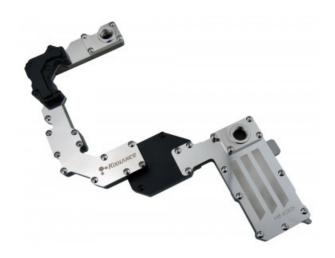
The MB-ASR3F water block is designed exclusively for the ASUS Rampage III Formula motherboard (not included). It liquid cools the northbridge chipset and other nearby components. Materials include copper with anti-corrosive nickel plating, acetal body, and steel top cover. G 1/4 BSPP fitting threading.
