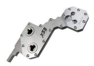
The MB-EVX58 water block is designed exclusively for the EVGA X58 SLI motherboard (132-BL-E758-TR and 132-BL-E758-A1). It liquid cools the northbridge and southbridge chipsets, along with nearby components. Materials include copper with anti-corrosive nickel plating and an acrylic top. G 1/4 BSPP fitting threading.
