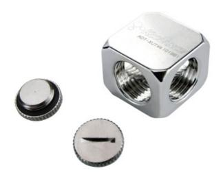
Extensible fitting bodies can be used to build such things as: splitters, tubing size adapters, drain valves, inline temperature sensors, elbow fittings, and more. This product has four G 1/4 BSPP (parallel) threads and includes two G 1/4 BSPP plugs. Made of nickel-plated brass.
