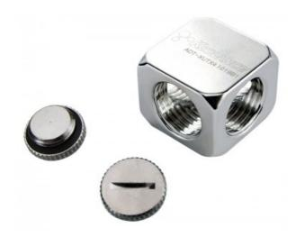
Extensible fitting bodies can be used to build such things as: splitters, tubing size adapters, drain valves, inline temperature sensors, elbow fittings, and more. This product has four G 1/4 BSPP (parallel) threads and includes two G 1/4 BSPP plugs. Made of nickel-plated brass.
