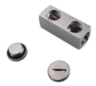
Extensible fitting bodies can be used to build such things as: splitters, tubing size adapters, drain valves, inline temperature sensors, elbow fittings, and more. This product has five G 1/4 BSPP (parallel) threads and includes two G 1/4 BSPP plugs. Made of nickel-plated brass.
