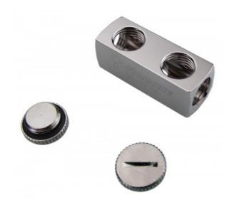
Extensible fitting bodies can be used to build such things as: splitters, tubing size adapters, drain valves, inline temperature sensors, elbow fittings, and more. This product has five G 1/4 BSPP (parallel) threads and includes two G 1/4 BSPP plugs. Made of nickel-plated brass.
