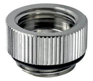
ADT-XMF is a Male-Female G 1/4 BSPP (parallel) thread coupler. Among various applications, it could be used as a spacer for obtaining extra fitting clearance. The body height, not including the male threading, is 7mm (1/4in).
