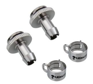
One pair of hose barb fittings for 1/4in (6mm) ID tubing. G 1/4 BSPP (parallel) thread. Nickel-plated brass with gasket, with hose clamp included.
