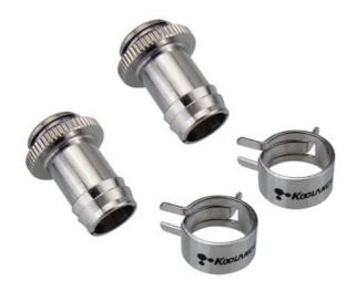
One pair of hose barb fittings for 3/8in (10mm) ID tubing. G 1/4 BSPP (parallel) thread. Nickel-plated brass with gasket, with hose clamp included.
