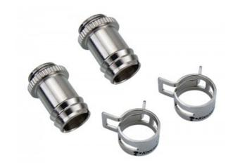
One pair of hose barb fittings for 1/2in (13mm) ID tubing. G 1/4 BSPP (parallel) thread. Nickel-plated brass with gasket. Hose clamp is included.
