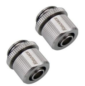
One pair of fittings for 1/4in (6mm) ID, 3/8in (10mm) OD tubing. G 1/4 BSPP (parallel) thread. Nickel-plated brass with compression fitting and gasket.
