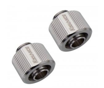
One pair of fittings for 3/8in (10mm) ID, 5/8in (16mm) OD tubing. G 1/4 BSPP (parallel) thread. Nickel-plated brass with compression fitting and gasket.
