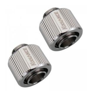
One pair of fittings for 1/2in (13mm) ID, 5/8in (16mm) OD tubing. G 1/4 BSPP (parallel) thread. Nickel-plated brass with compression fitting and gasket.
