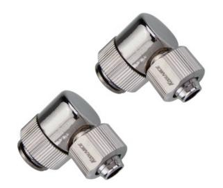
One pair of rotational angled fittings for 1/4in (6mm) ID, 3/8in (10mm) OD tubing. G 1/4 BSPP (parallel) thread. Nickel-plated brass with compression fitting and gasket.
