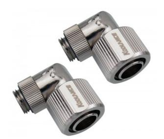
One pair of rotational angled fittings for 1/2in (13mm) ID, 5/8in (16mm) OD tubing. G 1/4 BSPP (parallel) thread. Nickel-plated brass with compression fitting and gasket.
