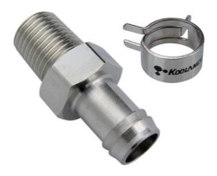
Single hose barb fitting for 3/8in (10mm) ID tubing. 1/4 NPT (tapered) thread. Hose clamp for 1/2in (13mm) OD included.
