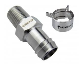
Single hose barb fitting for 1/2in (13mm) ID tubing. 1/4 NPT (tapered) thread. Hose clamp is included for 5/8in (16mm) OD tubing.
