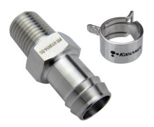
Single barb fitting for 1/2in (13mm) ID tubing. 1/4 NPT (tapered) thread. Spring clamp is included for 5/8in (16mm) OD tubing.
