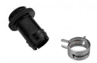
Single hose barb fitting for 3/8in (10mm) ID tubing. G 1/4 BSPP (parallel) thread. Includes hose clamp for 1/2in (13mm) OD tubing.
