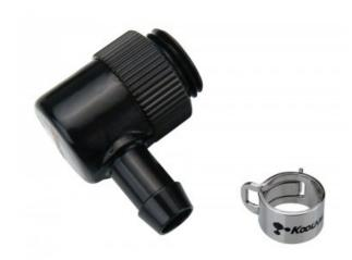
Single rotational angled fitting barb for 1/4in (6mm) ID tubing. G 1/4 BSPP (parallel) thread. Includes hose clamp for 3/8in (10mm) OD tubing.
