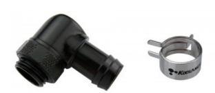
Single rotational angled fitting barb for 3/8in (10mm) ID tubing. G 1/4 BSPP (parallel) thread. Made of brass and includes hose clamp.
