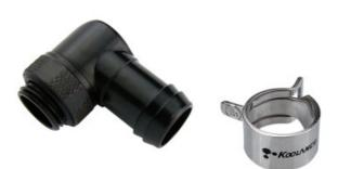
Single rotational angled fitting barb for 1/2in (13mm) ID tubing. G 1/4 BSPP (parallel) thread. Hose clamp included for 5/8in (16mm) OD tubing.
