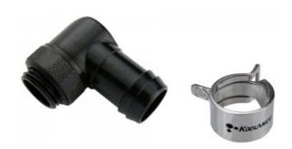
Single rotational angled fitting barb for 1/2in (13mm) ID tubing. G 1/4 BSPP (parallel) thread. Hose clamp included for 5/8in (16mm) OD tubing.
