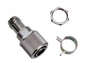
Single 3/8in (10mm) ID panel-mountable fitting. Compression fitting on one side, and hose barb on the other. Nickel-plated brass with gasket. Hose clamp and hex nut are included.
