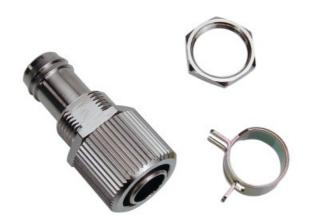
Single 3/8in (10mm) ID panel-mountable fitting. Compression fitting on one side, and hose barb on the other. Nickel-plated brass with gasket. Hose clamp and hex nut are included.
