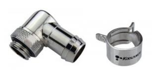
Single rotational angled fitting barb for 1/2in (13mm) ID tubing. G 1/4 BSPP (parallel) thread. Hose clamp included for 5/8in (16mm) OD tubing.
