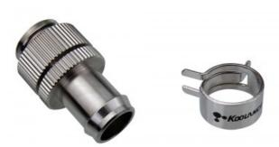
Single hose barb fitting for 3/8in (10mm) ID tubing. This fitting swivels to relieve hose stress and accidental loosening. To tighten or untighten, simply push in on the fitting and twist. G 1/4 BSPP (parallel) thread. Hose clamp included for 1/2in (13mm) OD tubing.
