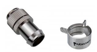
Single hose barb fitting for 1/2in (13mm) ID tubing. This fitting swivels to relieve hose stress and accidental loosening. To tighten or untighten, simply push in on the fitting and twist. G 1/4 BSPP (parallel) thread. Hose clamp included for 5/8in (16mm).
