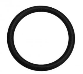
This is the most commonly used size of EPDM o-ring for Koolance G 1/4 BSPP fitting thread collars. 15.98mm outer diameter, 1.78mm thickness.
