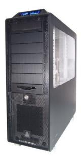
Get the maximum amount of space for large single or dual CPU systems with the PC3-736, which provides support for motherboards up to 12" x 13" (30.5cm x 33cm).
