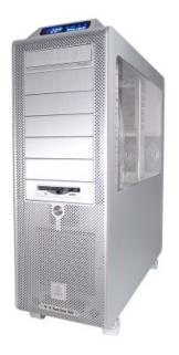
Get the maximum amount of space for large single or dual CPU systems with the PC3-736, which provides support for motherboards up to 12" x 13" (30.5cm x 33cm).
