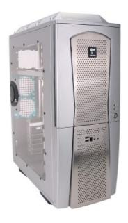
What does it take to reach 1000W of heat dissipation? The PC4-1000 series provides the first 1kW liquid cooling solution by Koolance. In this new generation, performance is accelerated with over three times the coolant flow rate of previous dual-pump systems (8.5 L/min, 2.25 GPM), a triple 120mm fan heat exchanger, and updated electronics.
