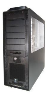
The PC5-1300 series offers heat dissipation of up to 1300W using a Koolance pre-installed quad-120mm fan heat exchanger. There is no pump included with this system, allowing you to choose among Koolance's RP-1000, PMP-450, PMP-400, or anything else! (Note: The RP-1000 is the reservoir, pump, and electronic control unit used in the Koolance PC4-1000 series system.)
