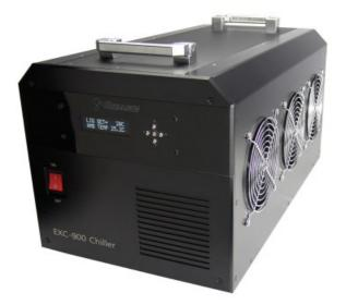
Koolance's EXC-900 is a compressor-refrigerant recirculating liquid chiller rated at 900W, or 3071 BTU/hr (@25°C liquid & ambient). Chiller control is based on one of four configurable temperature set-points, including the option to lock liquid to ambient for avoiding condensation or to an external K-type thermocouple sensor (not included).
