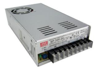
This is a power supply and wiring kit to power the Koolance <u>EXC-450</u> or <u>VLX-450</u> chillers from an AC outlet. DC and AC wires are included (AC plug is for North American outlets). The power supply is auto-switching, 100-240VAC 50/60Hz input to 24VDC output. It is rated to 312W, with PFC, and is CE and UL labeled. The size is approximately 9in x 4.5in x 2in (230mm x 115mm x 50mm).
