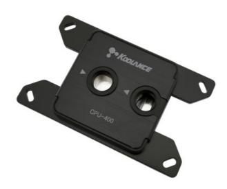
Koolance's CPU-400 features record-breaking thermal performance with a microfin nickel-plated copper cold plate, acetal top, and rugged steel mounting bracket. Standard G 1/4 BSPP threading will accept any Koolance fitting diameter up to 19mm (3/4in) OD compression style. Please select the desired fitting type for this base model (it does not include fittings). The CPU-400A supports most boards using the following processors:
