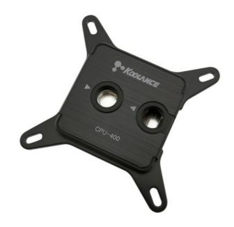
Koolance's CPU-400 features record-breaking thermal performance with a microfin nickel-plated copper cold plate, acetal top, and rugged steel mounting bracket. Standard G 1/4 BSPP threading will accept any Koolance fitting diameter up to 19mm (3/4in) OD compression style. Please select the desired fitting type for this base model (it does not include fittings). The CPU-400I supports most boards using the following processors:
