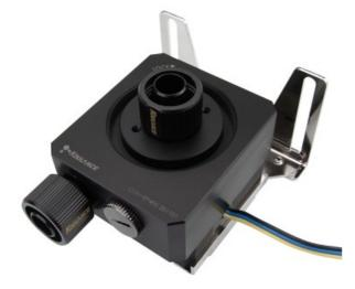
COV-RP400 is an acetal fitting and reservoir base for the Koolance <u>PMP-400</u> pump. Pump, reservoir, and fittings are sold separately. Along with enabling the use of any G 1/4 BSPP (parallel) thread fitting style and diameter, it allows flow to be specifically directed for increased pump performance or broader chassis integration. Fitting base, mounting bracket, coupler for 60mm OD reservoirs, socket plug, and mounting hardware is included.
