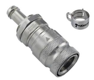
Koolance patented quick disconnect no-spill coupling with automatic shutoff. 6mm (1/4in) ID female panel-mountable barb fitting with spring clamp for 10mm (3/8in) OD. It will only fit a Koolance QD2H male quick disconnect.
