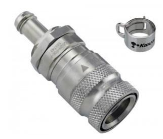
Koolance patented quick disconnect no-spill coupling with automatic shutoff. 6mm (1/4in) ID female panel-mountable hose barb with clamp for 10mm (3/8in) OD. It will only fit a Koolance QD2H male quick disconnect.
